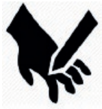
Pinch Point Warning
