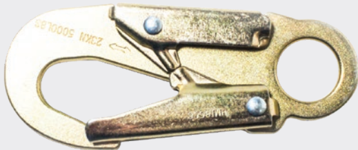
HMI8556 - Double Locking Snap Length: 140 mm (5-1/2 in) · Width: 57 mm (2-1/4 in) Working Load Limit: 2,267 kg (5,000 lb)
